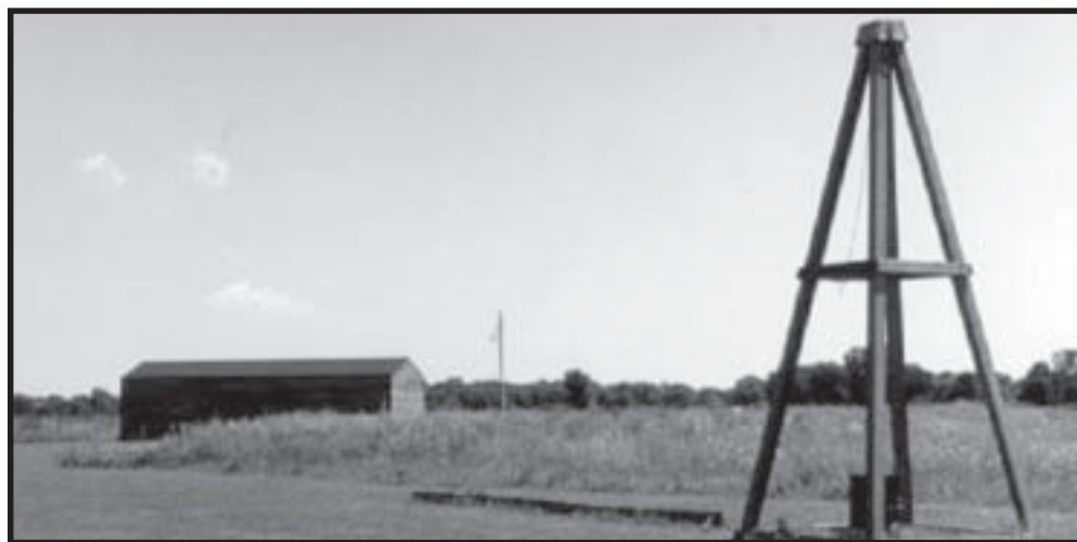
A view of the Wrights' monorail and catapult tower replicas-- the forerunner of catapults used on modern aircraft carriers.
