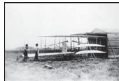
Wright Flyer III at the 1905 hangar. Note that elevators had to be removed for the airplane to fit.
