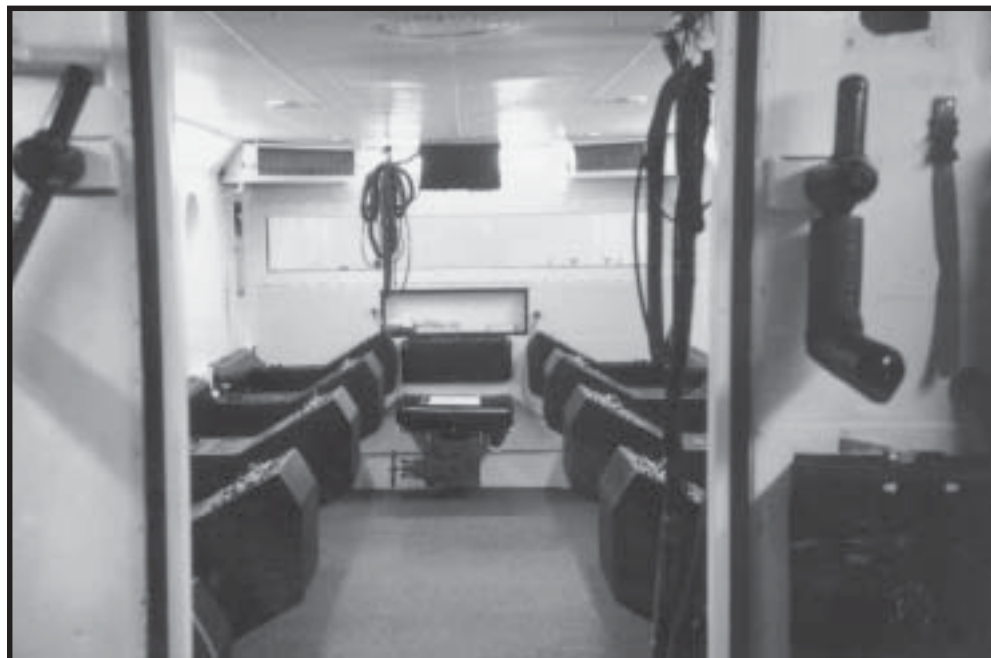
The Hypobaric (Altitude) Chamber, showing the inner room with sixteen student stations, used for demonstrating hypoxia and sudden decompression.
