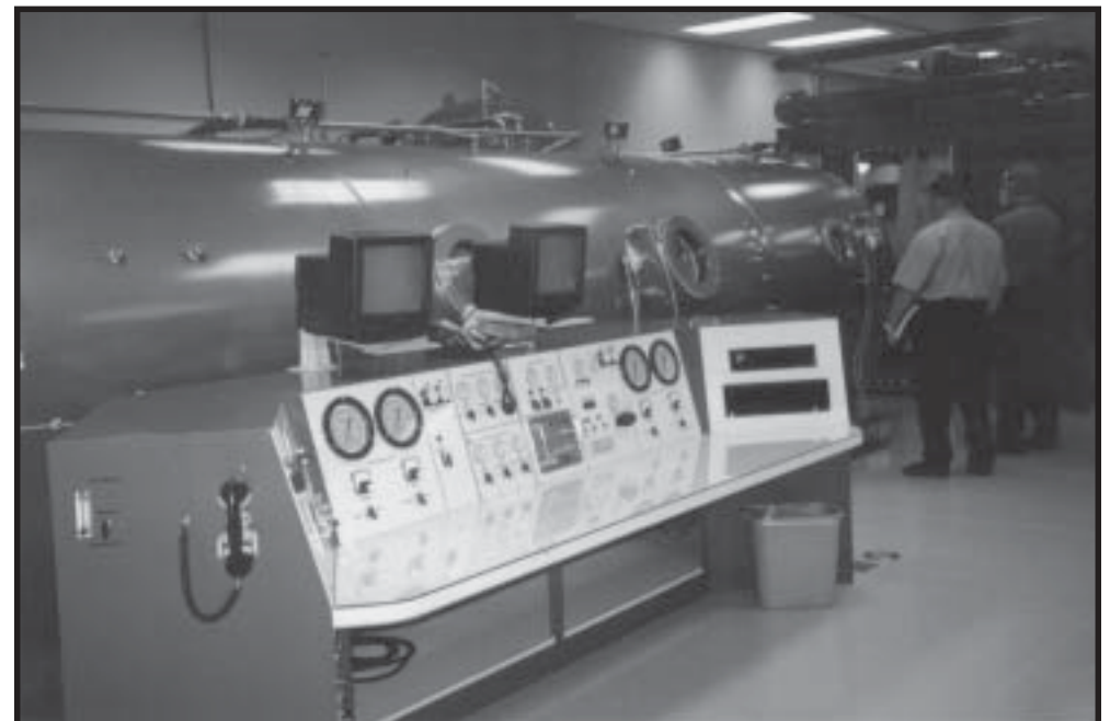
The Hyperbaric (Dive) Chamber, used to treat decompression sickness and many other medical ailments.
