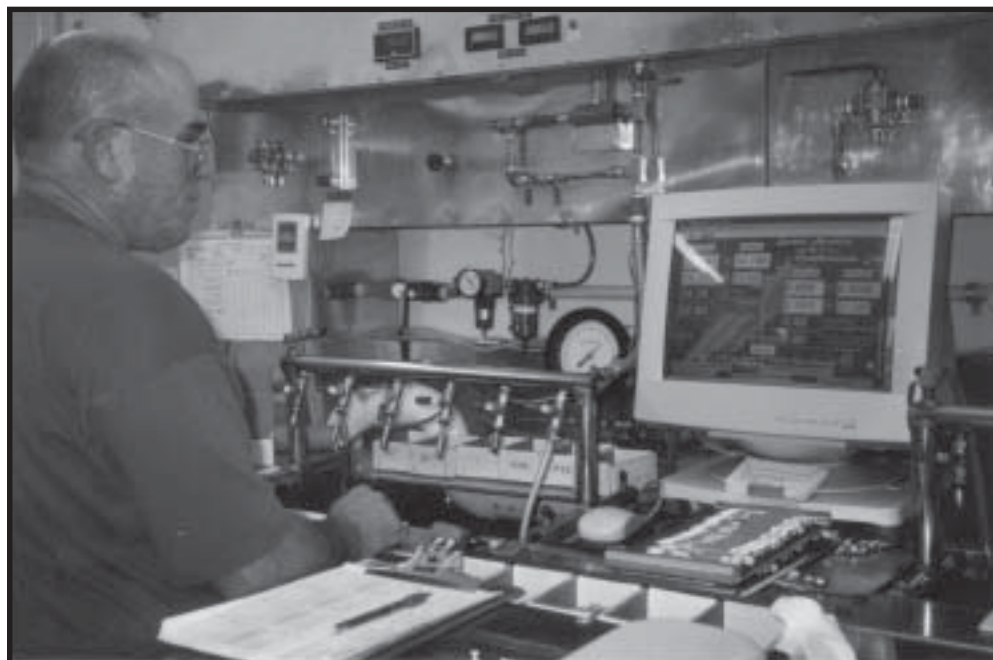
GAMI's super-precision flowbench, where GAMIjectors® are calibrated to one one-hundredth of a gallon per hour!
