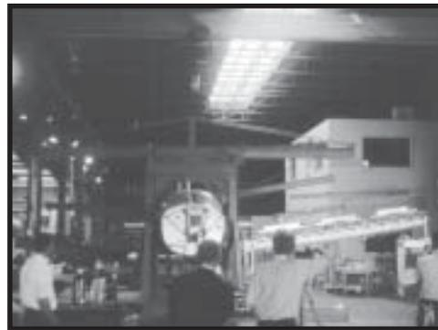
**A wing static test in process. A "whiffletree" arrangement of load attach points and lever arms is designed to allow wing loads to be applied with a single hydraulic cylinder, distributing the load spanwise per the FAA requirements.**
