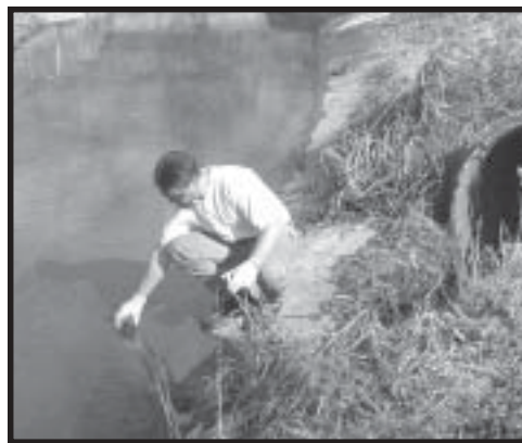
Jeff Phillips takes a water sample as part of a storm water pollution prevention plan.
