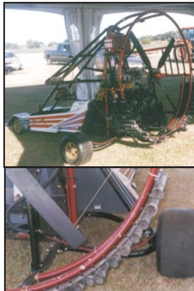
"Pyro Bill's" machine, with a go-cart-looking chassis, a Rotax 912 for power, strobes, colored lights, and a multitude of pyrotechnic tubes.
