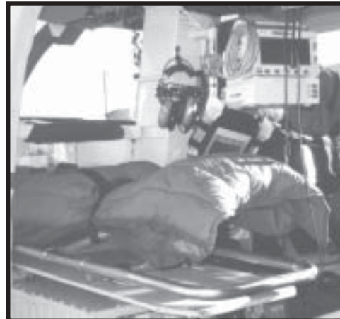
The patient station of the Bell 206-L, with a full complement of equipment to serve as a mini-emergency room in the air.
