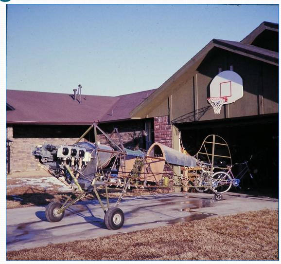
Here, I'm mocking up the exhaust headers using carboard tubes, welding rod around the curves, and plenty of tape.
