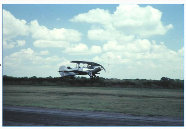
First approach! Round out the turn from downwind to final to keep the runway in sight. Raise the nose and the airport disappears under the long cowling. Maintain airspeed while looking for the runway edges in my peripheral vision. Begin the flare, power to idle, hold it off, hold it off, then, kiss, the wheels touch and it rolls straight!
