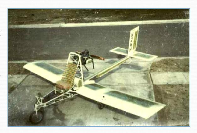
Problem was, it wouldn't fly with the little VW engine, so I borrowed a McCulloch 72-hp WWII target drone engine, doubling the horsepower and shaving about 40 lb off the empty weight.
